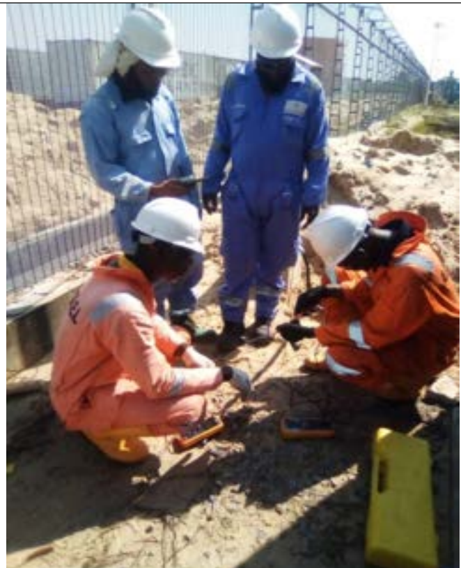
Fig 4.16: Insulation resistance testing of cables
